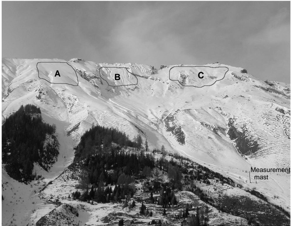
**Fig. 1.** Photograph of the Vallée de la Sionne test site showing the three possible release areas A, B and C and the 20 m high measurement mast. Photograph F. Dufour.
