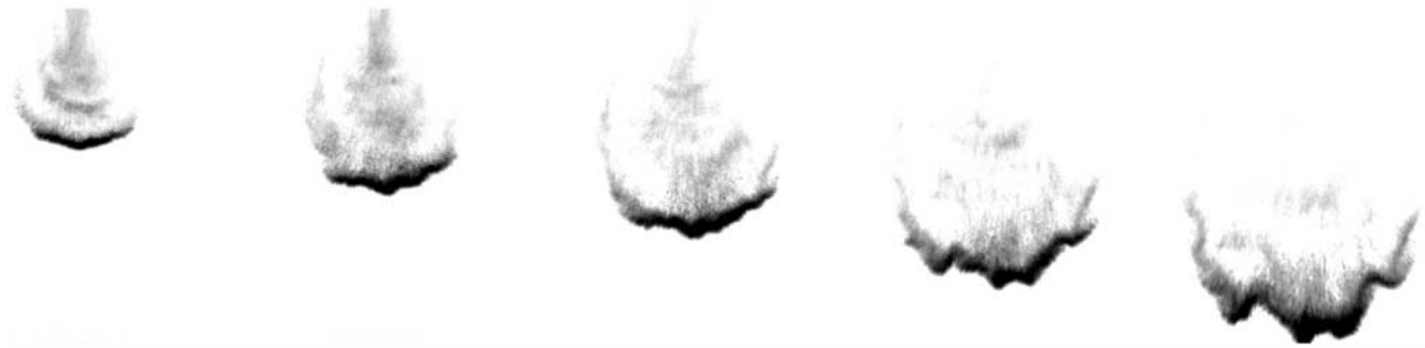
Figure 3. A 51 polystyrene current on a 51° slope showing front instability. The images are at three frame intervals, deinterlaced, and have an inverted color scheme with the background removed.
