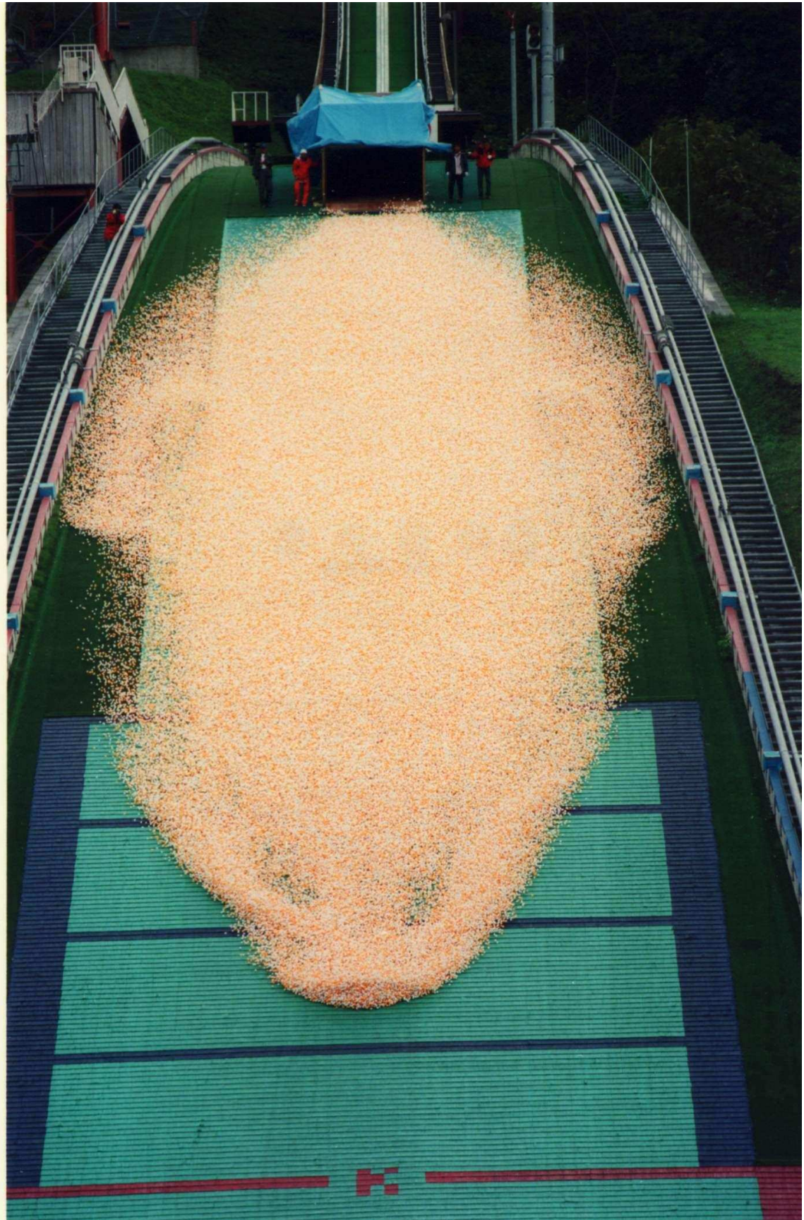
Figure 3: Front view of a 550,000 ball avalanche at the Miyanomori ski jump. The horizontal lines are 5 m apart and the lowest one is 90 m from the top of the landing slope.
